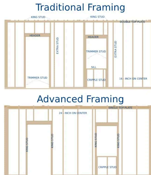
Figure 4. Comparison of Traditional vs. Advanced Wood Framing Layouts 6
